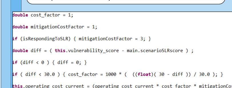
The code above shows that when the model's sea level rise score increases to within 30 points of a well's SLR vulnerability score, the cost of operating that well jumps by a factor of 1000 \* (1/30), or 333%. Operating costs for that well then increase linearly (by 333% per year) for 30 years.
