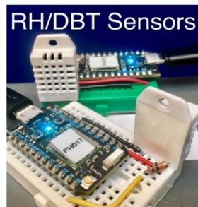
Figure 1. Arduino Protons, inexpensive RH/DBT distributive sensors used in both experiments.
