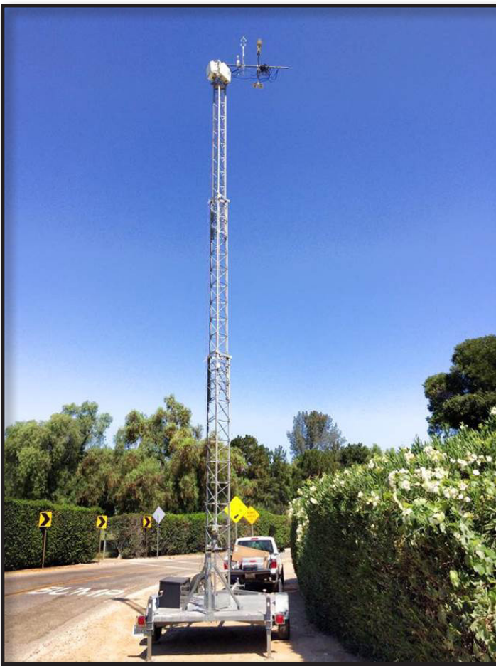
Picture left: Infrared gas analyzer and 3D sonic anemometer mounted to tower and moved throughout the landscape to measure the evaporative fraction lost to develop a relationship between satellite derived greenness (NDVI) and evaporative fraction. Pictured right: examples of air temperature sensors, called iButtons, that will be deployed throughout eight US metropolitan areas.
