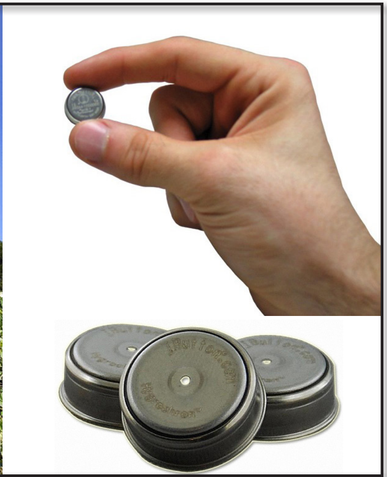
Picture left: Infrared gas analyzer and 3D sonic anemometer mounted to tower and moved throughout the landscape to measure the evaporative fraction lost to develop a relationship between satellite derived greenness (NDVI) and evaporative fraction. Pictured right: examples of air temperature sensors, called iButtons, that will be deployed throughout eight US metropolitan areas.
