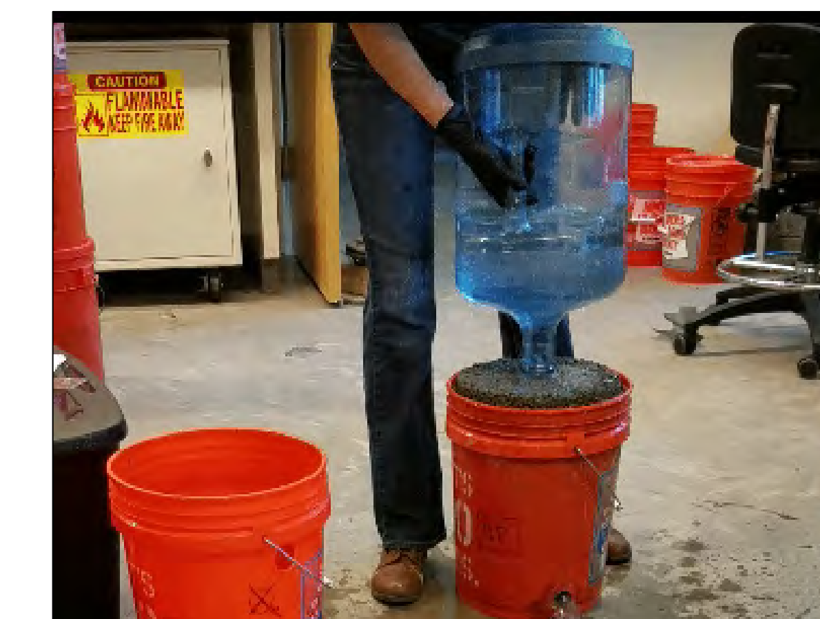
Figure 9 PeP filtration (left). Tested to effectively infiltrate 5 gallons of water in 66 seconds. Measured to infiltrate at a minimum flow rate of 17.5 in 3 /s. Test limited by outlet of containing bottle and effluent fluid exit area. Sand particles and debris did not affect infiltration rate. Strong thunderstorms drop 1-2" of rain. A 24 in 2 section of PeP is capable of infiltrating 2,376 in 3 volume of water in 2.26 minutes.
