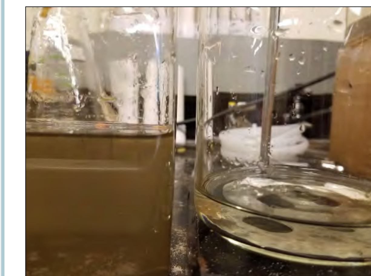
Figure 10 Raw untreated street runoff (left) and passively filtered water (right). Untreated storm water measured to have a turbidity of 50 NTU and geo-filtered storm water has a turbidity of 5 NTU. Geo-filtration layers were as follows: 25 g of MnO mixed sand, 5 g of GAC, 25 g of MnO sand, and 5 g of GAC. Columns measured 1.25" in diameter.
