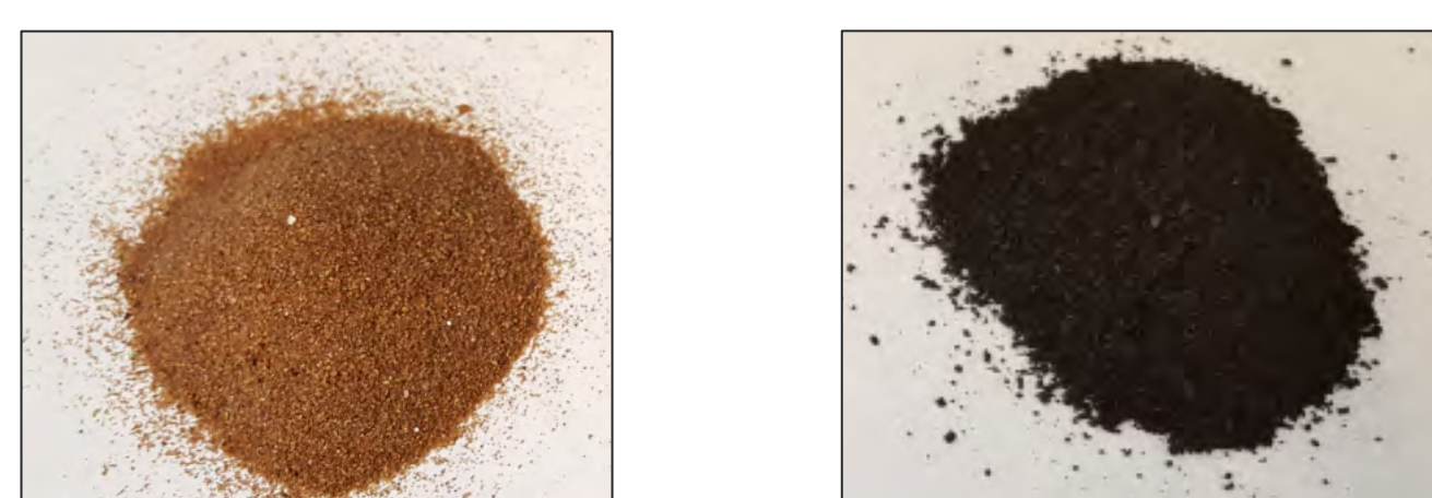
Figure 1 Synthesized Manganese Oxide Coated Sand (above left) and Granular Activated Carbon (above right).
