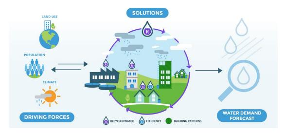
The <u>Integrated Urban Water Model (IUWM)</u> is a high level planning tool that allows urban planners and water managers to consider potable water savings of indoor and outdoor conservation measures, and alternative water sources such as graywater, stormwater, and reclaimed water. IUWM primarily projects water demands and revenue for municipal water providers through a combination of mass balance and empirical relationships.
